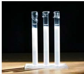
Fig. 3. Stability of emulsified fuel in according with the lapse of time.
