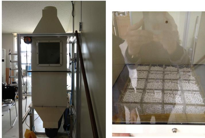
Fig. 3. Experimental equipment for wind tunnel and CO<sub>2</sub> filter module.
