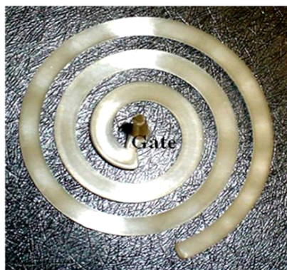
Fig. 2. Photo of injection molded specimen showing the flow mark.
