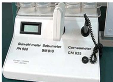
Fig. 4. Corneometer CM825 (Moisture Meter)
