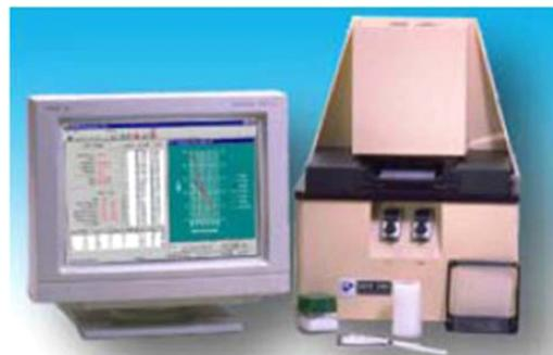
Fig. 1. SPF 290S Analyser: to evaluate SPF activity of in-vitro method.
