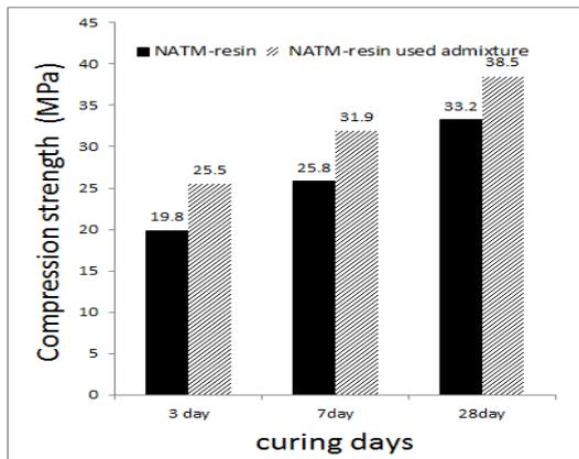
Fig. 4. Compression strength as a function of curing days by admixture of shrinkage compensating concrete in NATM-resin.
