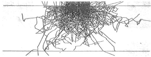
Fig. 2. Propagation pattern of photons(number of photons, 100) in scattering media. ( $\mu_s = 25.0 \text{ mm}^{-1}$ ,  $\mu_a = 3.0 \text{ mm}^{-1}$ ,  $z = 1.0 \text{ mm}$ ) by Roulette in Monte Carlo simulation.
