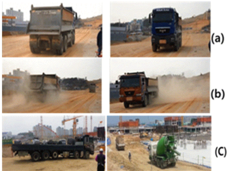
Fig. 7. Comparison of dust generation by 25ton vans after 2 days of spraying[(a) Dust suppressant spray area, (b)simple watering, (c) various field tests].
